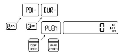
**STEP 2:** At the **PLEN** prompt, enter the length in current units you would like your pulse to be on. You can set the pulse to be on for a set length.
