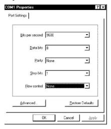
The next step is to set it so that when you look at data from the NS-60, it will display correctly on the screen. If you do not do this step the NS-60 will print all data on the same line on the screen.
